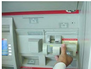
Skimmer being installed on front of existing bank card slot.
