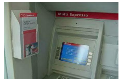
The camera shown installed and ready to capture PINs by looking down on the keypad as you enter number
