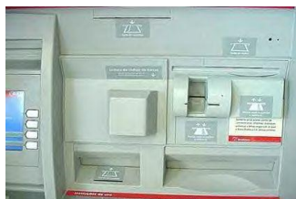
The equipment as it appears installed over the normal ATM bank slot.
